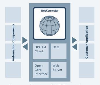
As a process data gateway, the WebConnector is the link between the web client and the automation environment
